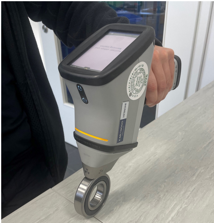
Non-destructive analysis of a rolling bearing with the X-MET8000 XRF handheld device
